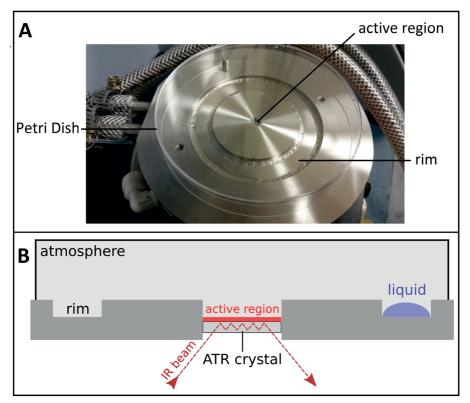
*Fig. 2.* FTIR spectrometer. (*A*) Photograph of the rim and active region of the measuring chamber, covered by a Petri dish to create closed and controlled environment. (*B*) Liquids (PFO and water) were placed either directly on the ATR crystal or in the surrounding rim.
