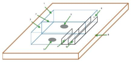
*Fig. 1.* Scheme of the chamber used in the first experiment. 1. Chamber B; 2. Chamber A; 3. IOL; 4. PFO dispensary dish injection site/dish; 5. Water dispensary dish injection site/dish; 6. Water-only dispensary dish injection site/dish; 7. Chamber divider; 8. Cooling/heating plate.
